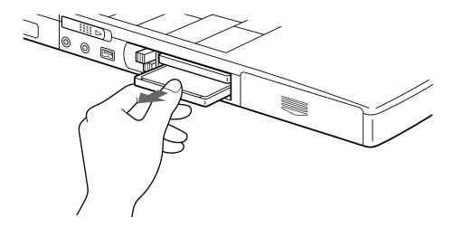
3 Insert the PC card into the PC card slot, front label facing up. Gently push the card into the slot until the card is fixed into the connector. The release button comes out.
