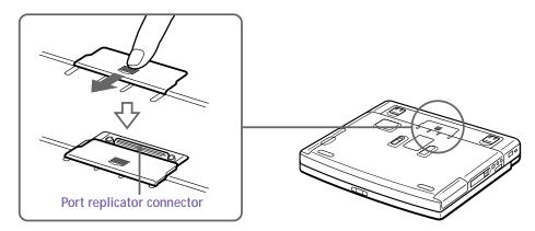
Attach the bottom of the computer to the port replicator connector until it clicks.
