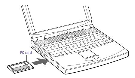
Do not force a card into the slot. It may damage the connector pins. If you have difficulty inserting a card, check that you are inserting the card with the correct orientation. See the manual that came with your PC card for more information on use.
