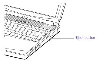
Place a DVD-ROM/CD-ROM in the tray with the label side facing up. For DVD-ROMs, which can be played on both sides, the side of the disc facing up is the side that plays. Push the disc onto the hub until the disc clicks into place.
