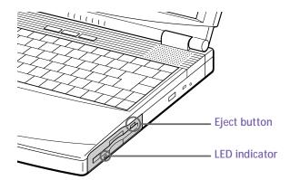
Do not press the Eject button when the LED indicator is turned on. Otherwise, data may be lost.
