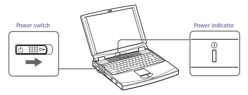
If you hold the power switch in the On position for more than four seconds, the computer turns off.
