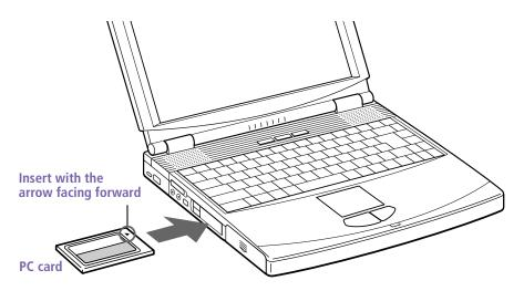
Do not force a card into the slot. It may damage the connector pins. If you have difficulty inserting a card, check that you are inserting the card with the correct orientation. See the manual that came with your PC card for more information on use.
