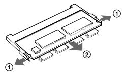
Pull the tabs in the direction of the arrows. The memory module is released.
