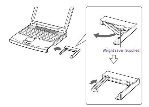
3 Manually lock the weight saver's RELEASE lever.
