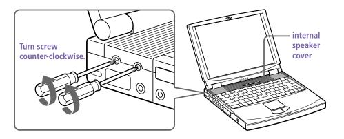
4 Slide the internal speaker cover to the right, then lift it away from the computer. Be careful not to detach the cable when lifting the cover.
