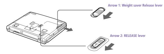
2 After removing the weight saver, pull out the weight saver's hinged arm and fold it into the weight saver.
