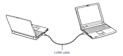
i.LINK cables compatible with your VAIO Notebook computer include cables with the following part numbers: VMC-IL4415 (a 1.5 meter cable with a 4-pin connector at each end), VMC-IL4435 (a 3.5 meter cable with a 4-pin connector at each end), VMC-IL4615 (a 1.5 meter cable with a 4-pin connector at one end and a 6-pin connector at the other), and VMC-IL4635 (a 3.5 meter cable with a 4-pin connector at one end and a 6-pin connector at the other).
