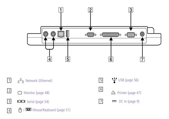
The port replicator can be powered only with an AC power adapter. Do not remove the AC adapter from the port replicator or the AC outlet while using the port replicator; this may cause data damage or hardware malfunctions.
