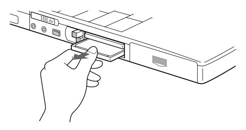
3 Insert the PC card into the PC card slot, front label facing up. Gently push the card into the slot until the card is fixed into the connector. The release button comes out.
