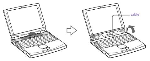
5 Unscrew above the keyboard, then gently lift the keyboard to stand it in the slot under the hole where the screw goes. Be careful not to detach the cable when lifting the keyboard.
