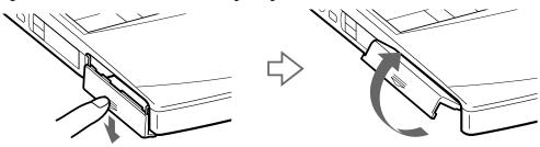
2 Insert the battery pack into the battery bay on the left side of the computer.
