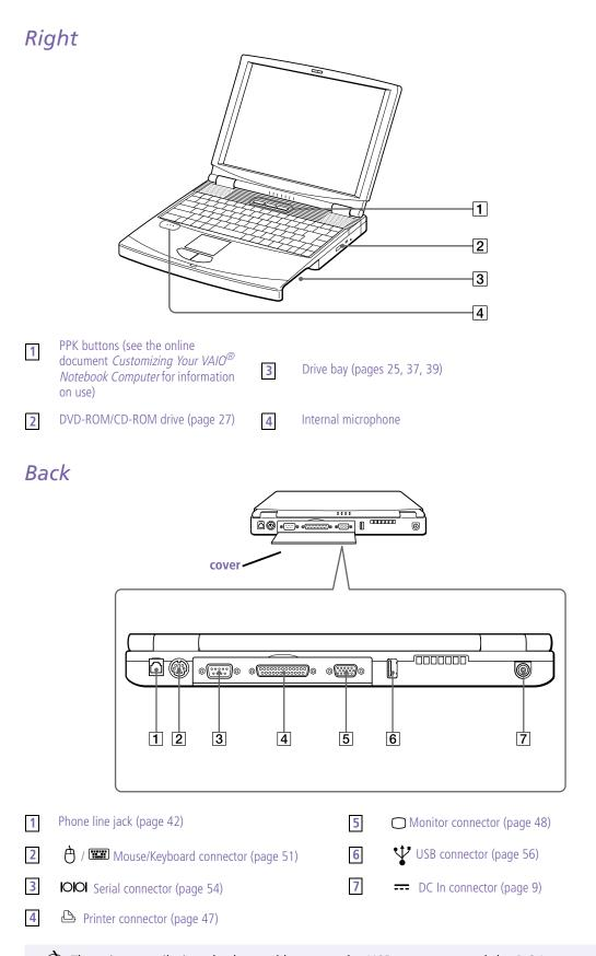
There is a ventilation slot located between the USB connector and the DC In connector. Do not cover the ventilation slot when your computer is on.
