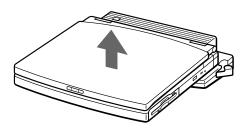
4 Close the port replicator connector cover on the bottom of your computer.
