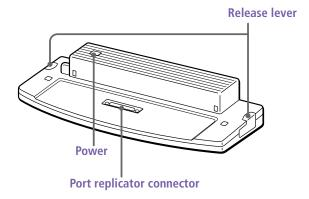
5 Turn on the computer. To remove your computer from the port replicator when the power is off
