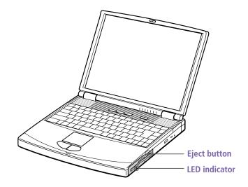
Do not press the Eject button when the LED indicator is turned on. Otherwise, data may be lost.
