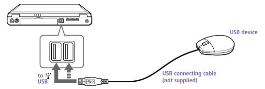
You can use the optional Sony USB mouse PCGA-UMS1 with this computer. The USB mouse software driver is preinstalled in the computer. Therefore you only need to plug the USB mouse into the USB connector.
