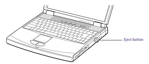
Place a DVD-ROM/CD-ROM in the tray with the label side facing up. For DVD-ROMs, which can be played on both sides, the side of the disc facing up is the side that plays. Push the disc onto the hub until the disc clicks into place.
