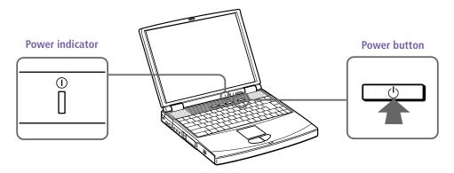
If you hold the power button in the On position for more than four seconds, the computer turns off.
