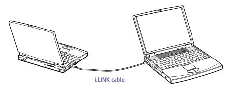
i.LINK cables compatible with your VAIO notebook computer include cables with the following part numbers: VMC-IL4415 (a 1.5-meter cable with a 4-pin connector at each end), VMC-IL4435 (a 3.5-meter cable with a 4-pin connector at each end), VMC-IL4615 (a 1.5 meter-cable with a 4-pin connector at one end and a 6-pin connector at the other), and VMC-IL4635 (a 3.5-meter cable with a 4-pin connector at one end and a 6-pin connector at the other).
