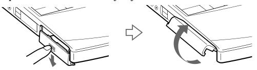
Insert the battery pack into the battery bay on the left side of the computer.
