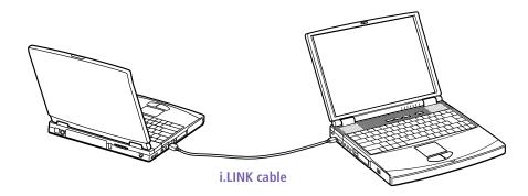
i.LINK cables compatible with your VAIO notebook include cables with the following part numbers: VMC-IL4415 (a 1.5-meter cable with a 4-pin connector at each end), VMC-IL4615 (a 1.5 meter-cable with a 4-pin connector at one end and a 6-pin connector at the other), and VMC-IL4408A (a 0.8-meter cable with a 4-pin connector at each end).
