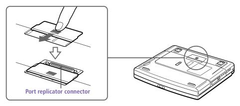
3 Attach the bottom of the computer to the port replicator connector until it clicks.
