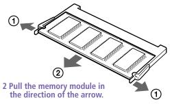
1 Pull the tabs in the direction of the arrows. The memory module is released.
