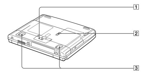
1 Port replicator connector cover 2 Multipurpose bay RELEASE lever 3 Tilt stands
