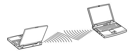
Infrared communication capability can be turned on and off. By default, it is disabled when your system is shipped. Use the infrared icon in the Windows Control Panel to enable/disable infrared communication.
