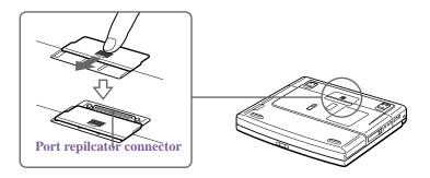
3 Attach the bottom of the computer to the port replicator connector until it clicks.
