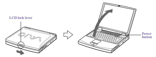
2 Press the power button on top of the computer until the green power indicator light turns on.
