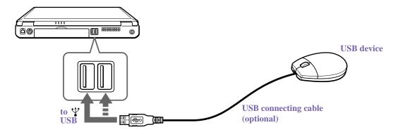
You can use the optional Sony USB mouse PCGA-UMS1 series with this computer. The USB mouse software driver is preinstalled in the computer. Therefore, you only need to plug the USB mouse into the USB connector.
