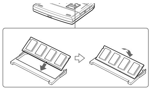
1 Slide the memory module into the slot.
