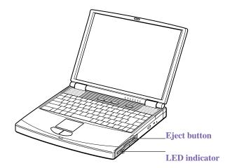
Do not push the eject button when the LED indicator is turned on. Otherwise, data maybe lost.
