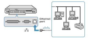
Warning: Only connect 10Base-T and 100Base-TX cables to the  $\frac{P}{d-d}$  Ethernet port. Do not connect any other type of network cable or any telephone line. Connecting cables other than those listed above may result in an electric current overload and could cause a malfunction, excessive heat, or fire in the port. To connect the unit to the network, contact your network administrator.
