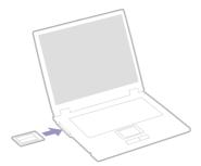
Gently push the PC Card slot into the connector. The PC Card is automatically detected by your system. The **Safely Remove Hardware** icon appears in the system tray.
