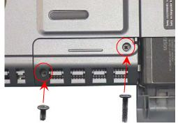
**Step 8.** Reinstall the two (2) screws previously removed.
