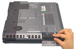
Step 2. Remove the Battery Pack.
