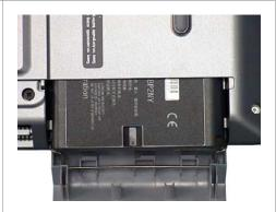
**Step 3.** Remove completely the battery pack from the computer and set aside.
