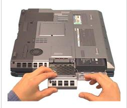
**Step 6.** Gently pull the original HDD Bay away from the computer as shown.
