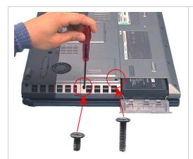
Step 4. Remove the HDD Bay.
