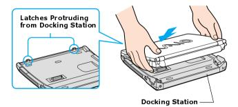
5 Push the two rear corners of the computer onto the docking station until it clicks into place and is securely fastened to the docking station.
