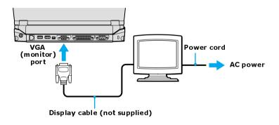
You cannot use the Monitor (VGA) port on your computer when the docking station is connected to the computer. Use the Monitor (VGA) port on the docking station instead.
