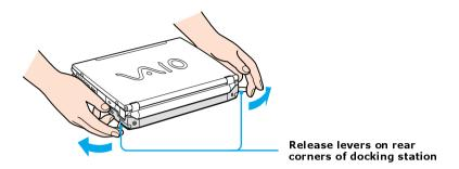
4 Lift the computer up and slightly back to disengage it from the two front latches of the docking station.
