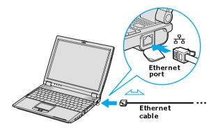
2 Plug one end of the Ethernet cable into your computer's Ethernet port  $\frac{9}{6.6}$  and the other into the network connection.
