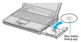
4 Press the disc onto the hub until the disc clicks securely into place.
