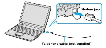
Your computer does not work with party lines, cannot be connected to a coinoperated telephone, and may not work with multiple telephone lines or a private branch exchange (PBX). Some of these connections may result in excess electrical current and could cause a malfunction in the internal modem.
