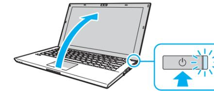
Press and hold down the power button until the power indicator light turns on.
