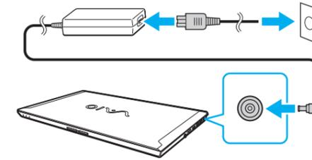
With the battery pack installed on your computer, plug the power cord and the AC adapter into an AC outlet and the computer.
