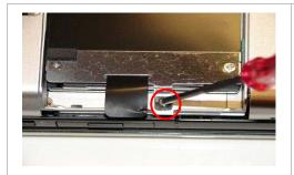
Step 10. Reinstall the one screw previously removed.
