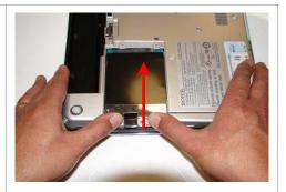
Step 9. Once hard drive is properly sitting its bay, carefully re-connect the hard drive to the connector by sliding the hard drive in the direction shown above.
