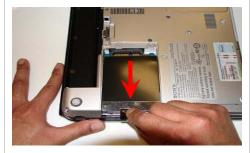
(HDD must be disconnected) Step 6. Locate the black plastic tab on the hard drive assembly and gently pull the original hard drive in the direction shown above.
