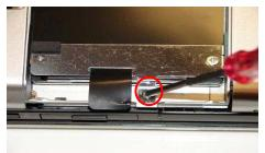
**Step 5.** Using the enclosed magnetic screwdriver, remove the one (1) screw securing the hard drive assembly.
