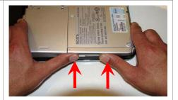
**Step 9.** To ensure proper assembly and connection, with even force push the ODD back into place.
