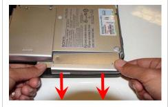
**Step 6.** With even force carefully remove the optical drive by pulling it away from the unit.
