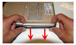
**Step 5.** To initiate the removal of the optical drive, slightly pull the optical drive door as shown in the picture.
