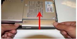
**Step 8.** Carefully slide the optical drive into the bay and back into place.
