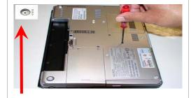
**Step 11.** Re-install the previously removed screw.
