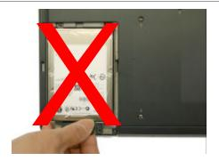
CAUTION: Do not pull the plastic tab upwards before releasing the hard drive from the connector!
