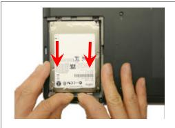
**Step 6.** With even force slide the HDD by pulling the plastic tab on the direction of the arrow. Some force may be needed to unlock the HDD from the connector.
