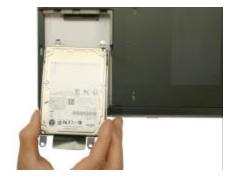
**Step 8.** Hold the new HDD by the edges and slide it inside the opening in an angle.
