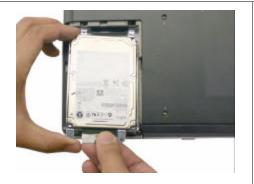
**Step 7.** Gently pull out the original HDD away from the computer as shown.
