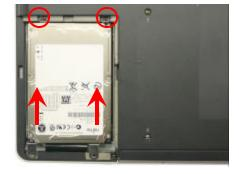
**Step 9.** Align the HDD with the connector and with even force push in the new HDD. Reinstall the two (2) previously removed screws.
