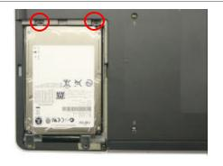
**Step 5.** Using the enclosed magnetic screwdriver, remove the two (2) screws as indicated in the picture.
