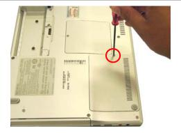
Step 11. Re-install the HDD cover.
