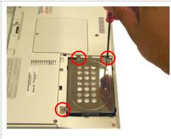
**Step 6.** Using the enclosed magnetic screwdriver, remove the three (3) screws securing the HDD assembly.
