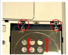
**Step 9.** Attach the HDD assembly to the HDD connector. Make sure the screw holes are aligned correctly.
