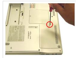
**Step 4.** Using the enclosed magnetic screwdriver, loosen the one screw securing the hard disk drive access cover.
