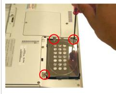
**Step 10.** Re-install the three (3) screws securing the HDD assembly in place.
