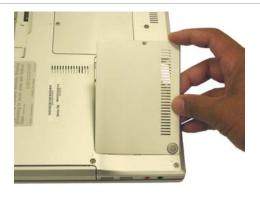
**Step 5.** To remove the HDD access cover, start by lifting from the side where the screw held it in place.
