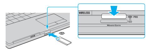
Be sure to hold the Memory Stick media with the arrow pointing in the correct direction as you insert it into the slot. To avoid damaging your computer or the Memory Stick media, do not force the Memory Stick media into the slot if you cannot insert it smoothly.
