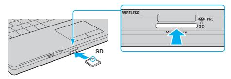
**3** Carefully slide the memory card into the slot until it clicks into place. Do not force the card into the slot.
