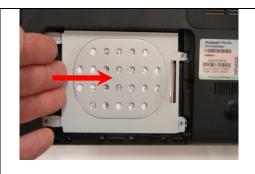
Step 15. Install the Hard Drive by sliding the assembly to the right. <u>Make sure the</u> screw holes align correctly.
