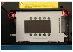
Step 5. Using the enclosed magnetic screwdriver, remove the two (2) screws securing the Hard Drive Assembly. <u>Put</u> aside the Hard Drive Screws to resecure the Hard Drive later in the procedure.
