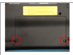
**Step 18.** Re-install the two (2) Hard Drive Door Screws to secure the Door.
