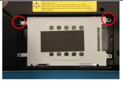
**Step 16.** Re-install the two (2) Hard Drive screws holding the Hard Drive Assembly in place.
