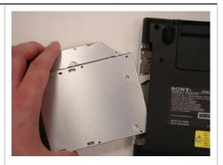
**Step 6.** Carefully remove the ODD Assembly from the unit.
