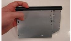
**Step 11.** Align the tabs on the Bezel with the tab holes located on the ODD. Carefully press the Bezel into place.
