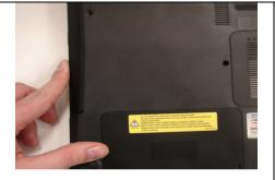
**Step 15.** Make sure the new ODD is seated flush on the edge of the computer.
