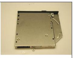
**NOTE:** After installation, all brackets should sit flush with the ODD. The stamped letters located on the brackets should all be facing the same direction.
