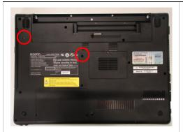
Step 4. Using the enclosed magnetic screwdriver, remove the two (2) screws securing the ODD Bay. <u>Put aside the ODD Bay screws to re-secure the ODD Bay later in the procedure.</u>
