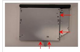
ODD Disassembly (Steps 7-9) Step 7. Identify the four (4) side screws that secure the ODD Brackets to the ODD.
