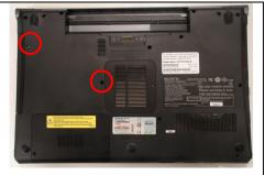
**Step 16.** Reinstall the two (2) ODD Bay screws to secure the ODD Drive Bay.
