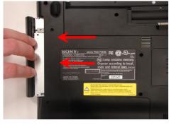
**Step 5.** Insert your fingers in the space between the ODD and the unit. Gently pull towards the Left to remove the ODD.
